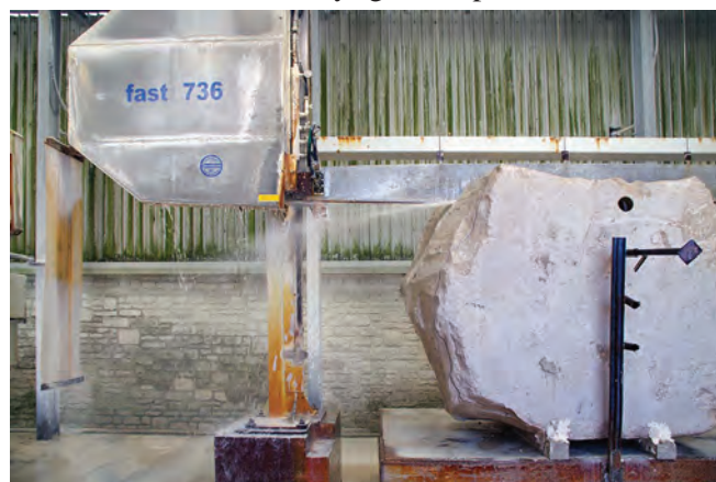
Front view of an initial cut Benetti horizontal chainsaw reducing blocks to manageable size; water is cascading off the cutter and stone dust jetting from the blade
